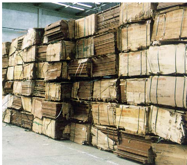
Plywood bundles that have broken out of packing that is insufficient for the weight of the bundles and bearers
